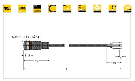
M12-Kupplung, gerade, 4-polig + PE
