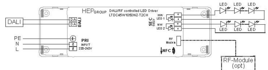
Cross-section area of conductor for input terminal block: 0.75-1.5 mm<sup>2</sup> (cord type at least H03VVH2-F),
