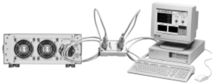
Fig.1-1 Connect the electronic load to PC
