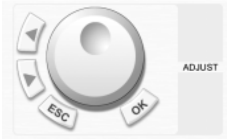
Fig.1-5 Rotary knob and function keys
