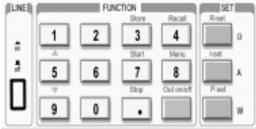
Fig.1-4 Keyboard of SSL KONSTANTER 32 EL Series DC electronic load
