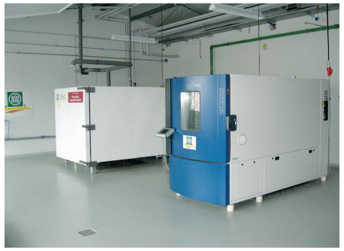
Figure 2: DLG test lab – two ammonia chambers
