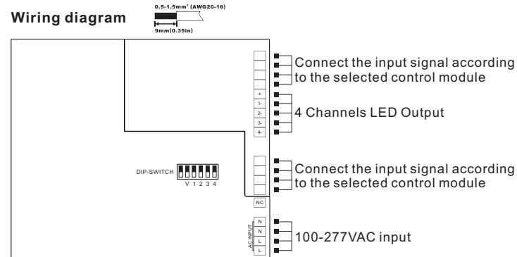
Note: for detailed wiring diagram, please refer to the user manual of corresponding control module.
