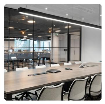
Ceiling rose: Matching luminaire's surface colour. Mediumpower current. 7110lm. 56W. 6kg. Binning initial <= MacAdam 3. IP20. Protection class I. CE, UKCA marking. Prüfzeichen: ENEC. IK02. 220-240V. 50-60 Hz. RG0 (EN62471). Luminous flux reduction up to 0,3%/1.000 operating hours. Nominal failure rate: 0,2%/1.000 operating hours. L85B10 (tq 25°C) = 50.000h. 5 years warranty. Manufacturer: Lightnet GmbH, ISO 9001:2015 and 50001:2018 certified.
