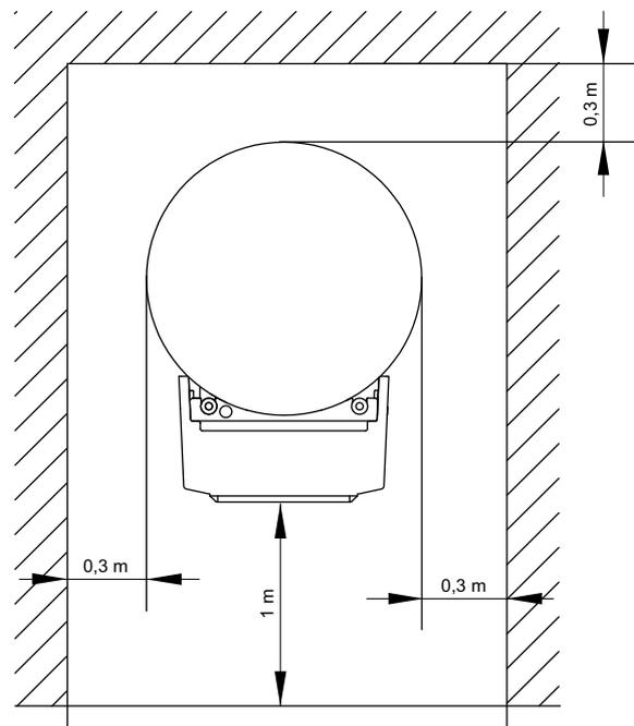
If the hydraulic tower is installed on an upper floor, the load-bearing capacity of the ceiling should be checked. On account of the acoustics, measures for isolating possible vibrations should also be very carefully planned. Installation on floors above wooden ceilings is not recommended.
