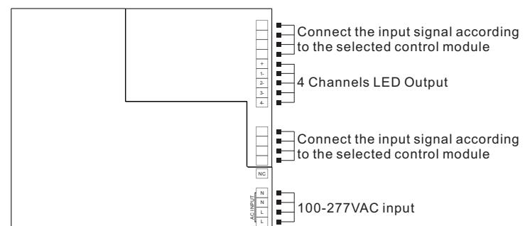
**Note:** for detailed wiring diagram, please refer to the user manual of corresponding control module.
