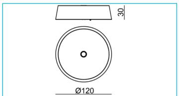
Housing Material Die-cast aluminium
