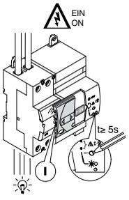
To configure the auxiliary contact, the slider must be moved left to position AUTO ON (1).
