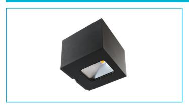
The square JABBAH uses integrated COB LEDs in warm white, emitting its light asymmetrically at an angle of 75° onto walls in a cone of illumination - in a simple variant providing 915 lumens, as an UP AND DOWN version providing a total of 1,850 lumens. In addition, the two-sided JABBAH can be dimmed to 60 % luminous flux using a dip switch, if a more subtle light is desired.
