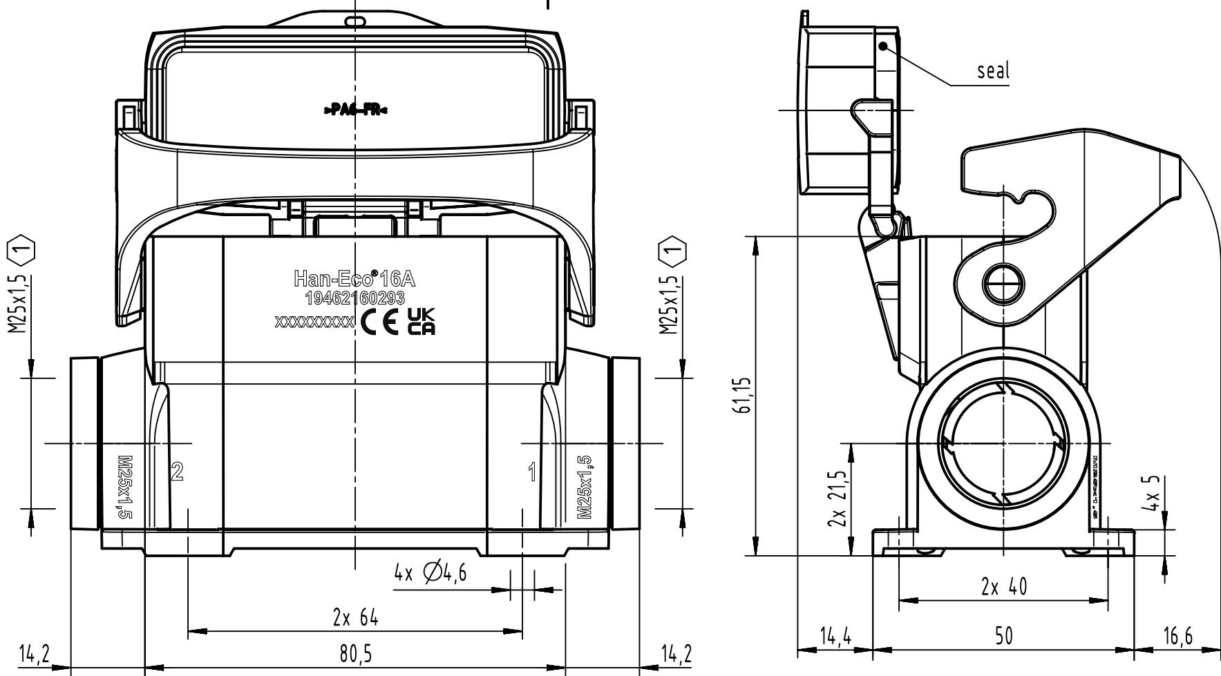
① tightening torque max. 10Nm
