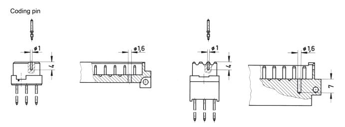
Drill out the male connector at pre-centered point according to the sketch. The coding pin can then be inserted into the corresponding cavity of the female connector by means of the insertion tool. This coding system is available only for the types D, E, F and interface connectors I.
