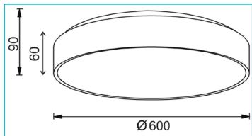
**Housing Material** Aluminium, Polycarbonate, Iron **Housing Color** Black **Housing Surface** Matt **Material of Lens** Acryl **Surface Structure of Lens** Satined
