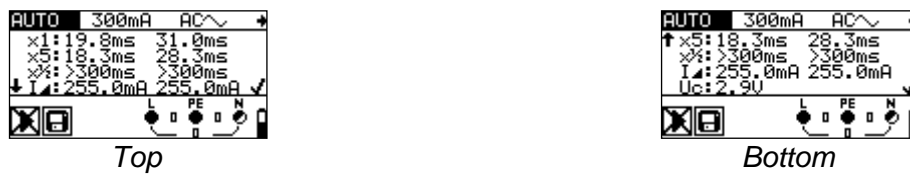
Figure 5.22: The "HELP" key toggles between the upper and the lower part of the result field.
