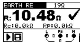
Figure 5.35: Example of an earthing resistance measurement
