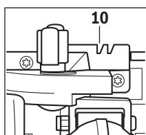
Use only cutting mark **10** when making a right-angled cut and a 45° cut with the guide rail.
