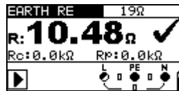
Figure 5.35: Example of an earthing resistance measurement
