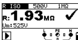
Figure 5.7: Example of an insulating resistance measurement
