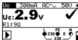
Figure 5.18: Example of a contact voltage measurement
