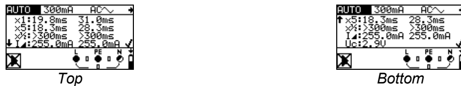
Figure 5.22: The "HELP" key toggles between the upper and the lower part of the result field.
