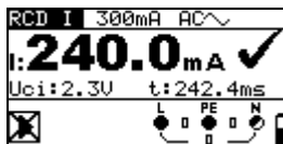
Figure 5.20: Example of a tripping current measurement
