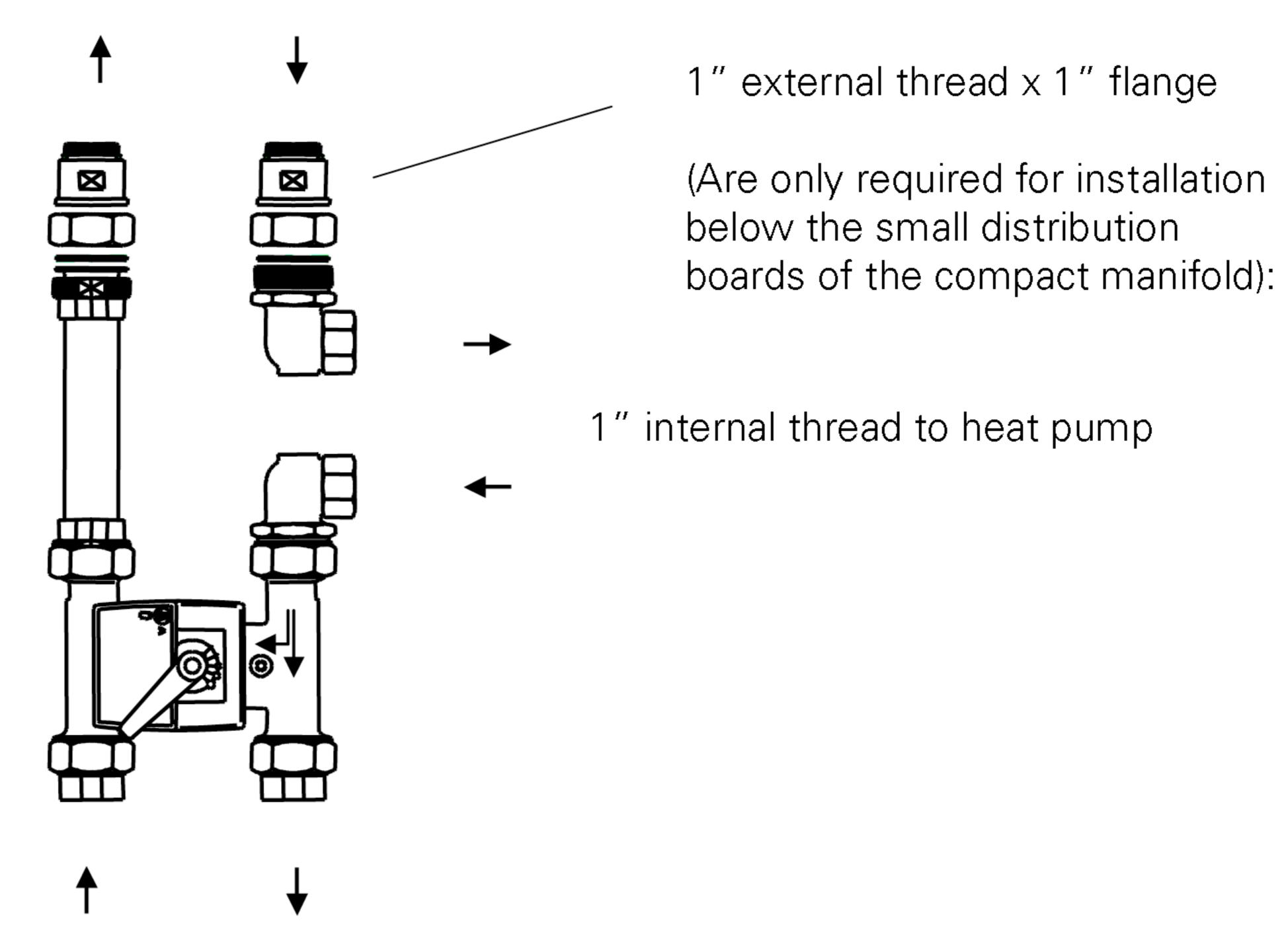
1" internal thread to alternative heat source (e.g. oil or gas boiler)
